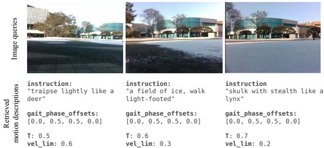
Fig. 6. LocoVLM successfully interprets the scenes in the form of RGB images and provides the robot with motion descriptors that are suitable for the observed scenes.
